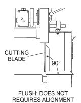
Figure 29. Cutting Head Alignment (Vertical)
